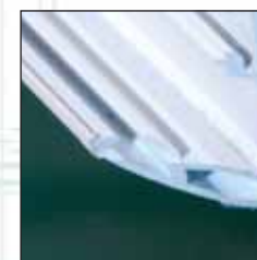
Removal of weld sprue area
