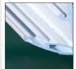
Removal of weld sprue area
